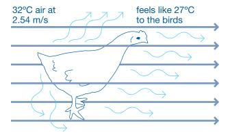
Birds can tolerate higher temperatures during the day if night time temperatures drop 14°C or more below daytime highs. During the cool night time birds can get rid of excess body heat built up during the day. Running fans to get air moving over the birds during the night can help by reducing the "effective" night time temperature. The birds then can start the next day fresh, which helps keep performance up and lessens the risk of possible mortalities if daytime temperatures are very high.
