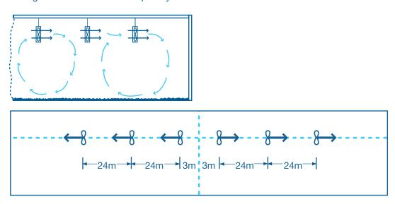
**Figure 24:** Typical installation details and air circulation pattern achieved by paddle stirring fans in a 12 m x 152 m poultry house
