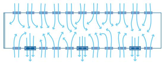
Minimum ventilation is timer-driven, and may be set to operate as little as one-half minute in five early in a growout or in very cold weather. As birds grow larger and/or weather warms, thermostats override the timer to provide an adequate ventilation rate.
