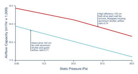
Figure 20: Fan Efficiency m³/hr/watt Comparison
