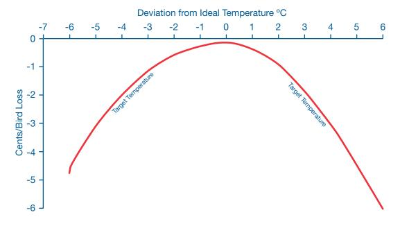
Being just a few degrees off target temperature in the growing phase can hurt grower income significantly. The above graph shows cents per bird differences in total returns for consistent on-target vs. off-target temperature control for non-brooding phase birds. Conditions: Broilers grown to 49 days, meat sold for \$0.89 per kg, no dockage for non-uniformity; feed costs \$278/tonne Starter, \$270/tonne Grower, \$258/tonne Finisher. Source: Veng, Hot climate ventilation.
