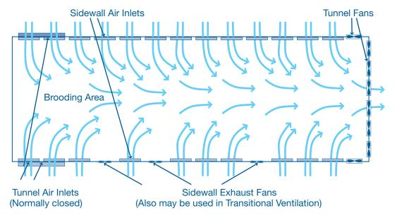
As with minimum ventilation, the air inlet area during transitional ventilation must be matched to the fan capacity used. Enough sidewall inlet area should be provided to operate at least half of the installed tunnel fans in the hybrid transitional mode without creating excessive static pressure. For most efficient operation, air inlets are controlled by static pressure-operated machines, as in minimum ventilation.
