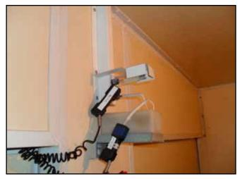
After positioning the calibration probe in the machine, allow sufficient time for the machine and sensors to stabilize. Typically this will take 30 minutes.
